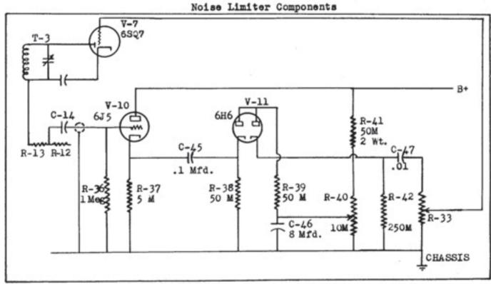
Schematic diagram illustrating Noise Limiter section of Circuit
