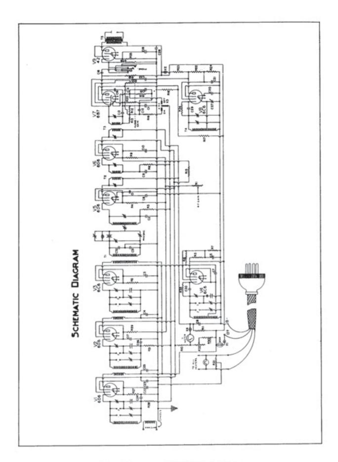
Circuit Diagram of HRO-M Radio Receiver
